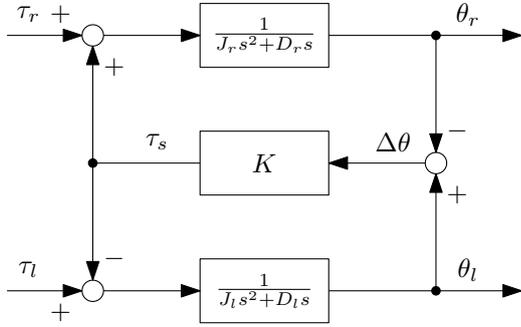
Figure 7: Block diagram of two-inertia system.
