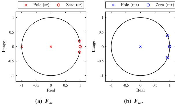
Figure 9: Poles and zeros of multirate feedforward controller  $F_{mr}$  and single-rate feedforward controller  $F_{sr}$  with unit circle on  $z$  plane.
