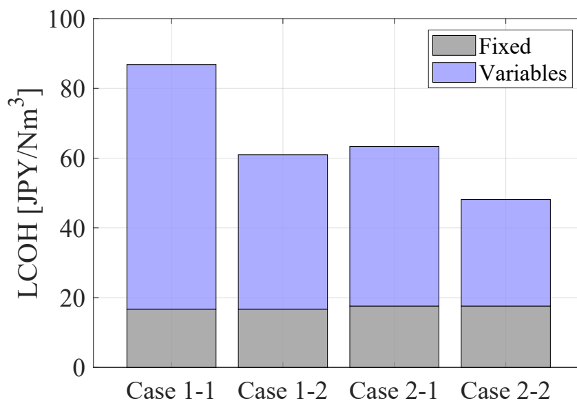
Figure 19. Comparison of LCOH between the Tokyo and Kyushu regions. The electrolyzer capacity factor is 50% in both cases.
